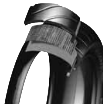
0° - STEEL BELTED TYRE WITH RADIAL CARCASS (90 DEGREES)
