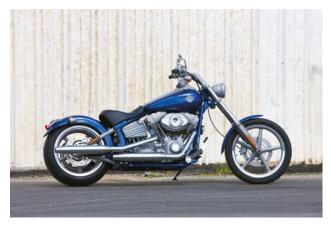
The Rocker offers authentic hard-tail chopper style with innovative ideas that could onlybe produced by Harley-Davidson. The Rockertail rear section mounts a wide fender directly to the swingarm, over a big 18-inch rear tyre. The Rocker rear fender and wheemove in unison as the Rockertail glides through 79mm of rear suspension
